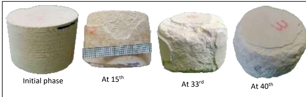
Figure 5. 2. 49 S3 specimen under magnesium sulfate salt solution
