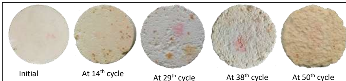
Figure 5. 2. 36 S3 specimen under sodium chloride salt solution
