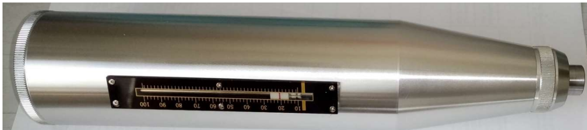
Figure 4. 3. 4 “VSYIQI” HT-75 brick rebound hammer
