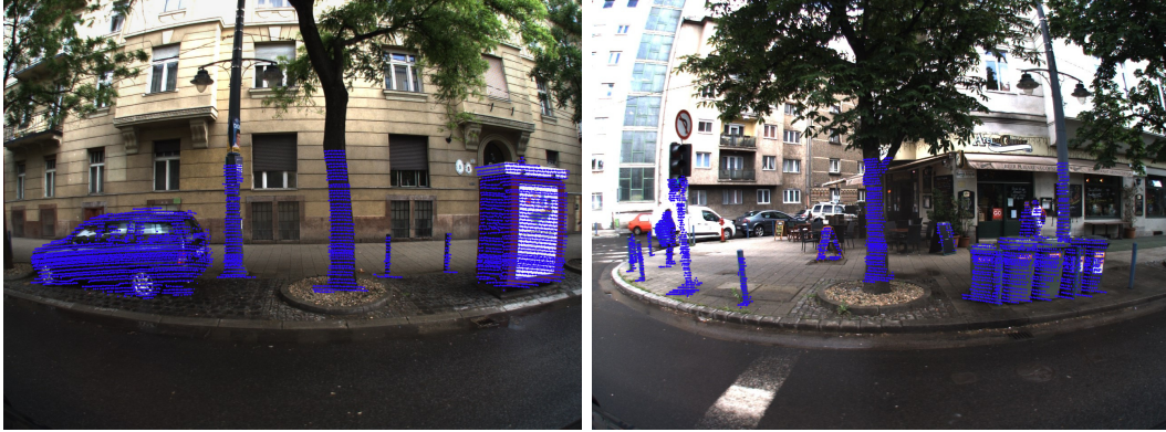
Figure 1.2: Projection results of the proposed target-less, automatic camera-Lidar calibration method [1].
