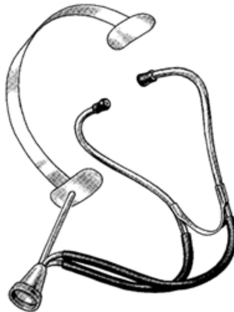
Figure 1.2: The DeLee-Hillis stethoscope (fetoscope) for fetal auscultation, keeping the hands of the obstetrician free during the examination.
