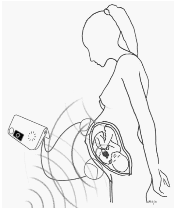
Figure 4.4: Sources of noise corrupting the low intensity fetal heart sound signal: noise from the mother (maternal heart and digestive sounds), noise from the fetus (hiccup, movements of the limbs) and noise from the environment. Courtesy of Julianna Ottlik.
