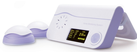
Figure 4.2: Phonocardiographic CTG device type Fetaphon-2000 TM enabling the home surveillance of the fetus.
