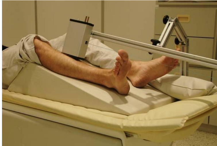
Figure 6.1 PC-MR-compatible mechanical stimulus presentation equipment in the 3 Tesla Philips Achieva scanner (Philips, Best, The Netherlands) room
