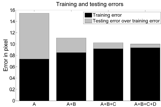
Figure 9: Training with speaker A, A and B, and so on, and always test by speaker E which is not involved in the training set.
