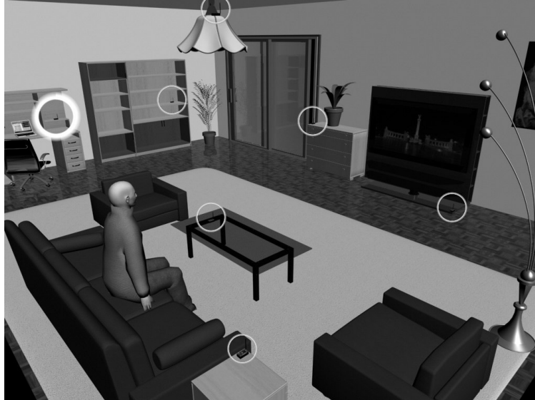
Figure 4.1. The room accommodating the patient. The CRUs and the G-CRU installed across the room are highlighted by the thin circles and the thick circle, respectively. The packet transmitted by the implant is received by multiple CRUs, which then cooperatively make the decision on the implant packet.
