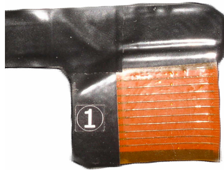
Figure 3.2. One of the four 9×9 element pads of the XSensor
