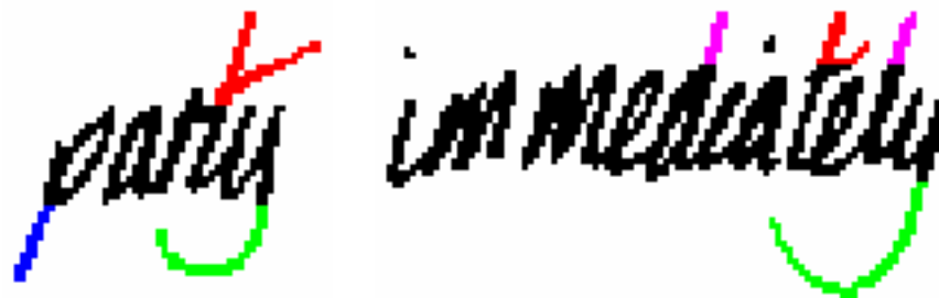
Figure 2.8. Feature maps showing different types of ascenders and descenders. Red and purple refer to normal and narrow ascenders, blue and green refer to narrow and wide descenders, respectively.
