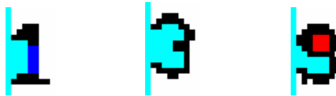
Figure 5.6. Sample feature maps. Right open holes and their auxiliary lines are shown in cyan, middle vertical line is shown in blue, and upper round hole is shown in red.
