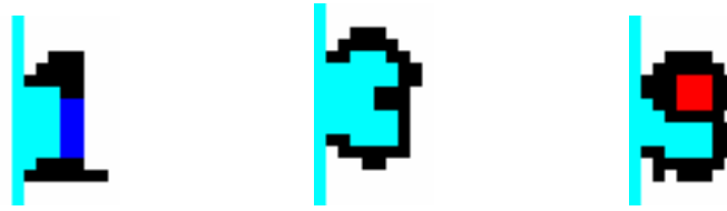
Figure 3.9. Sample feature maps. Right open holes and their auxiliary lines are shown in cyan, middle vertical line is shown in blue, and upper round hole is shown in red.
