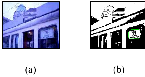
Figure 5.4. Sign localization on a tram. (a) Original input frame (b) Sign location on binarized input
