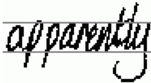
Figure 2.3. Computed baselines of the word ‘apparently’. Upper and lower baselines cut off ascenders and descenders (Section 2.7.3) respectively from the main word body.
