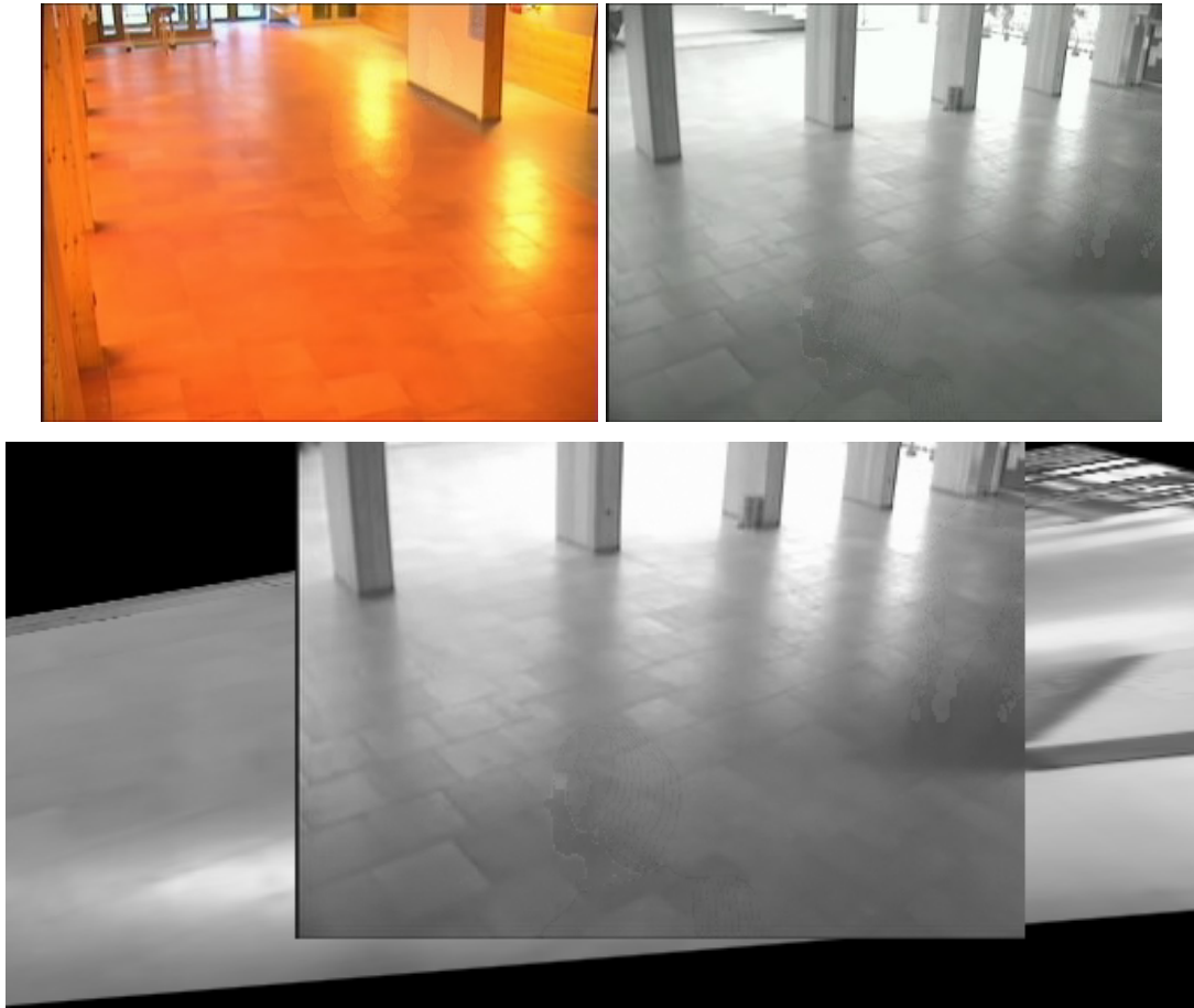
Figure 2-20. Alignment of views based on the detection of concurrently moving shadows.
