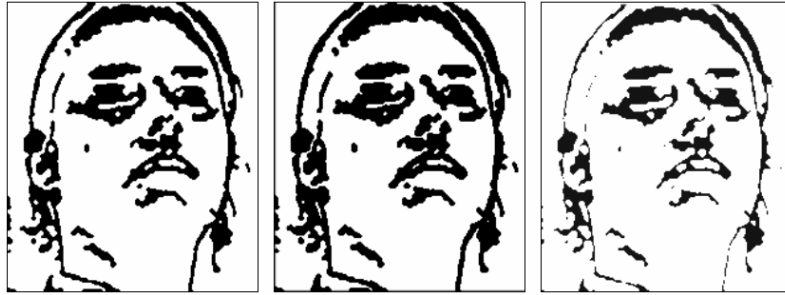
Figure 3-6. The input and outputs of Dilation and Erosion template operations
