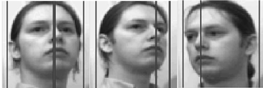
Figure 3-17. Results of ACE4K experiments of the face symmetry axis detection algorithm for faces in different poses
