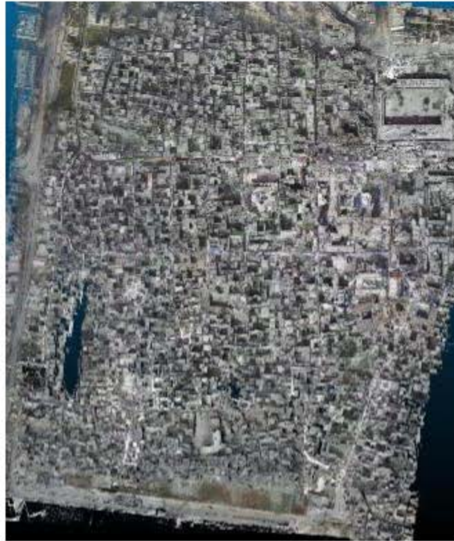
Fig. 68 The Drone-Point-Cloud after adding the data from the video, saved from Cloud.
