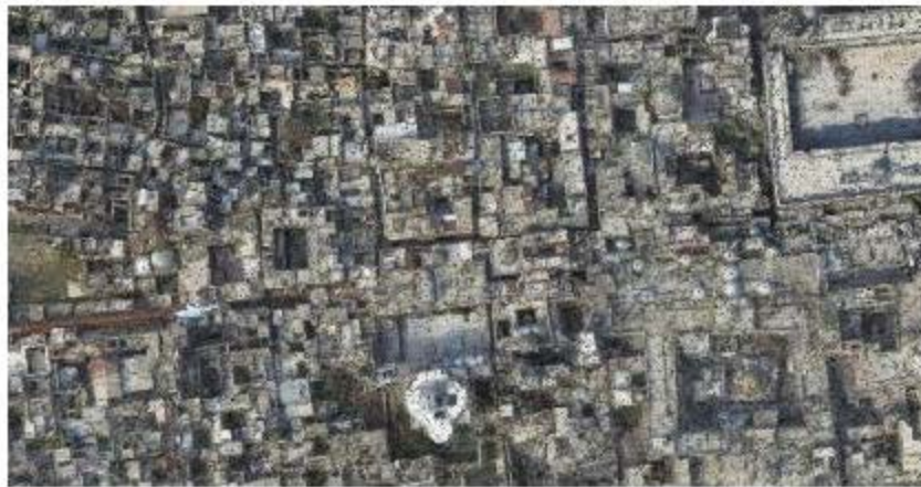
Fig. 58 A section of the resulted high-resolution point cloud in Agisoft Photoscan, by Orabi, 2023.
