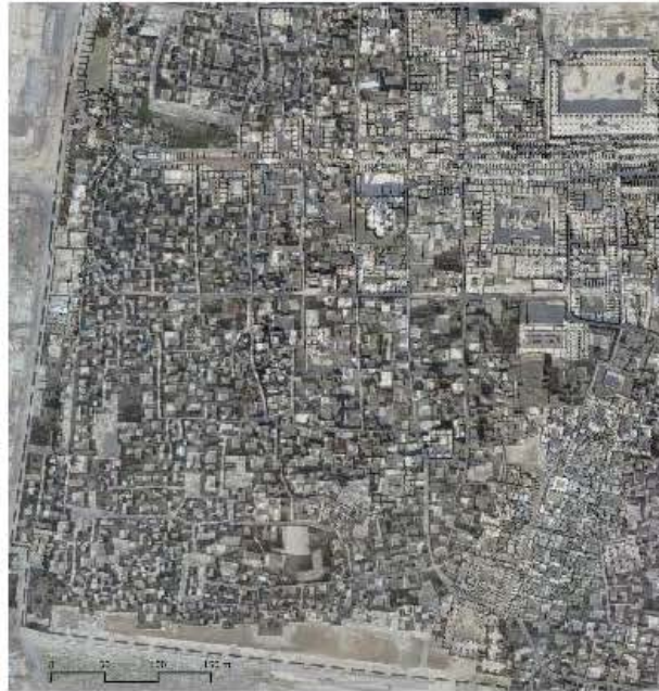
Fig. 43 The orthophoto from the survey overlaid with the AAE map, exported from QGIS, compiled by Orabi, 2023.
