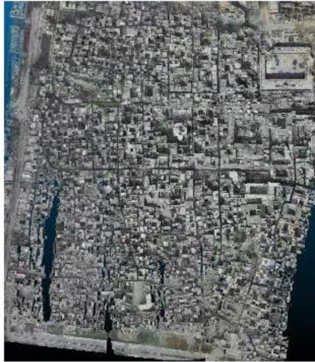
Fig. 59 The laser scan and the aerial photogrammetry (Photos and Video) combined in Cloud Compare, by Orabi, 2023.
